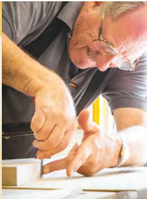
Another Japanese tool, this time a knife, whose high-carbon steel takes an excellent edge, and flat back suits it beautifully to cutting veneers following a deep guide
